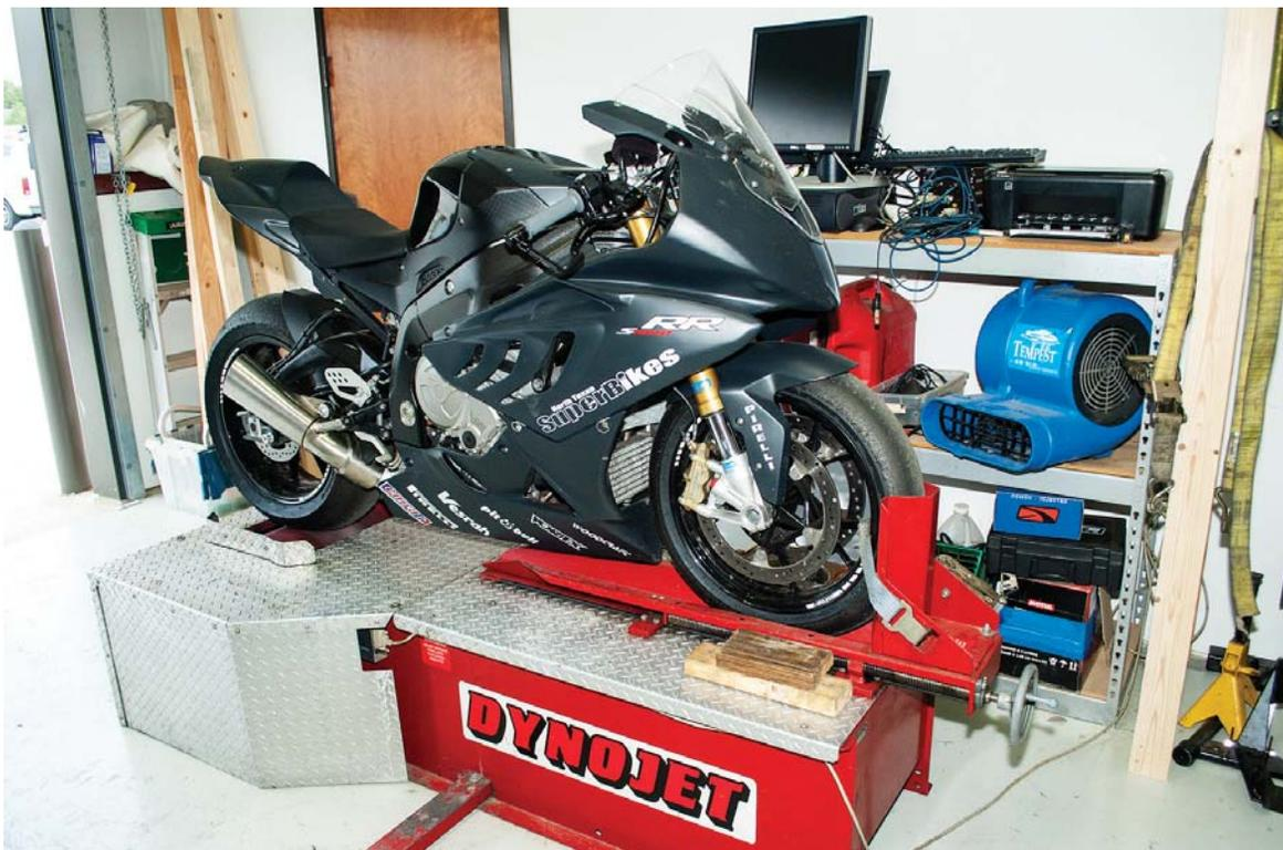
(Above) A Dynojet Model 250i dyno is used to diagnose problems, clean up fuel-injection mapping and reflash ECUs. (Right) The shop is an authorized sales and service center for Öhlins, Penske and Traxxion Dynamics. (Below) A 50-foot trailer allows the shop to offer arrive-and-ride at-track service plans to customers who do track days and race.
